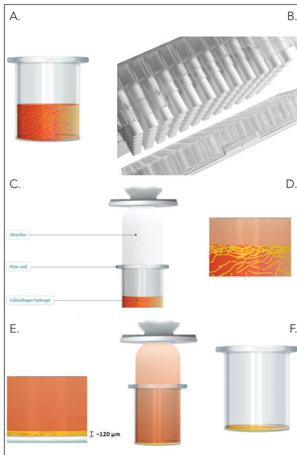
**Figure 1. Creation of 3-Dimensional Cell/Collagen Hydrogel using RAFT™ System.** (A) Cell/collagen mix dispensed to wells of 96-well plate. (B) 96-well RAFT plate containing individual sterile absorbers. (C) Absorber insertion into plate well. (D) Absorption of medium, concentrating collagen and cells to *in vivo* strength. (E) Completion of absorption process creating 120 µm thick hydrogel. (F) Removal of absorber prior to dispense of fresh cell medium.
